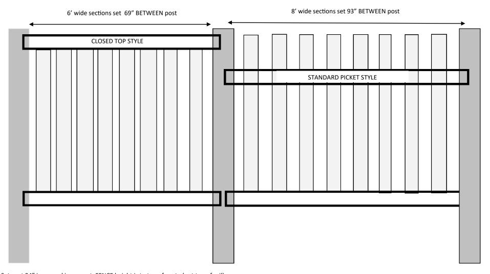
Set post 24" in ground in cement FENCE height is to top of post. (not top of rail)
